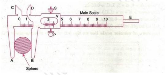
Vernier callipers measuring diameter of a sphere.
