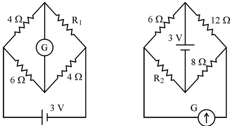
Define the term current sensitivity of a galvanometer. In the circuits shown in the figures, the galvanometer shows no deflection in each case. Find the ratio of  $R_1$  and  $R_2$ .
