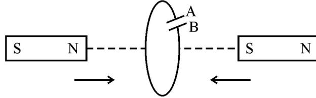
In the figure given, mark the polarity of plates A and B of a capacitor when the magnets are quickly moved towards the coil.
