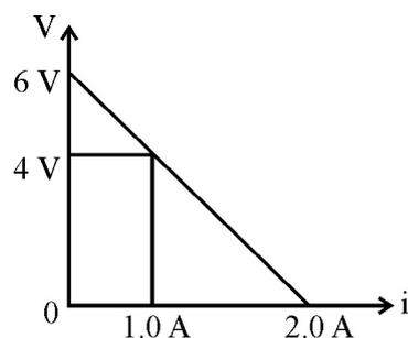
The figure shows a plot of terminal voltage 'V' versus the current 'i' of a given cell. Calculate from the graph (a) emf of the cell and (b) internal resistance of the cell.
